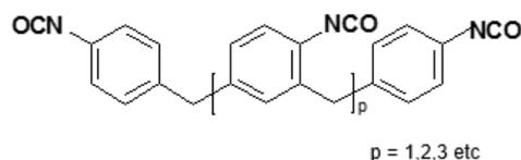
Figure 3. Molecular structure of monomeric and polymeric MDI.
