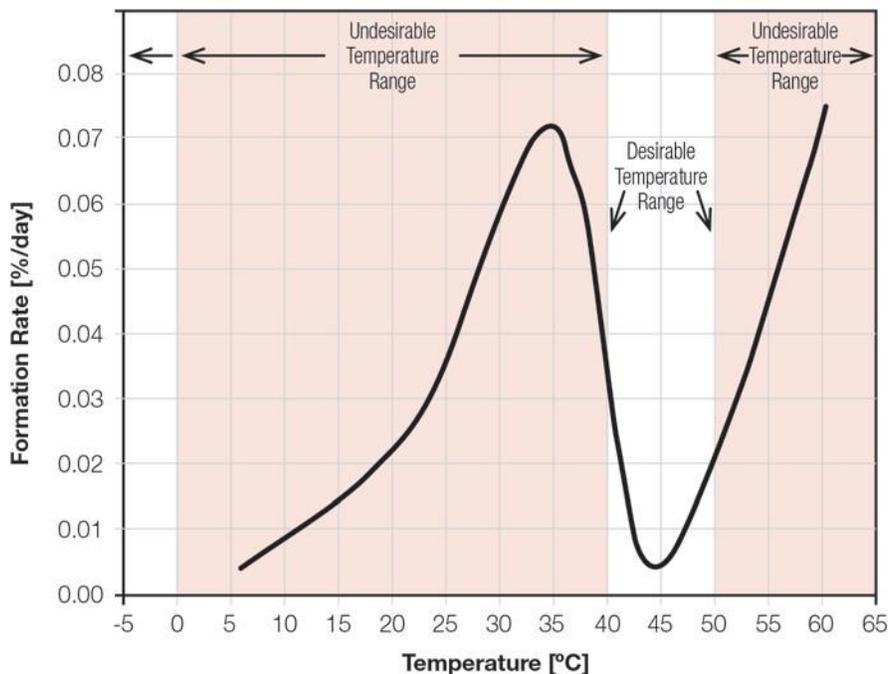
Figure 4. Lupurate® M: Rate of dimer formation as a function of storage temperature.
