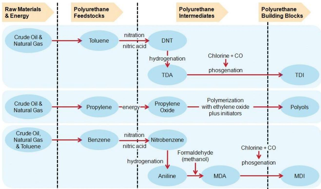
Figure 2. Process summary for the production of polyurethane building blocks.
